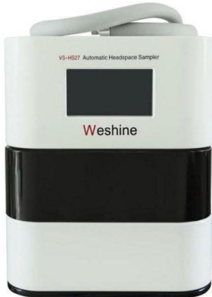
The Autosampler can extract the gases from the insulating oils, and transmit the gases by carrier gas to the **Gas Chromatography Calibration** Columns. It has the function of heating and shocking, instead of the manual oscillator.
